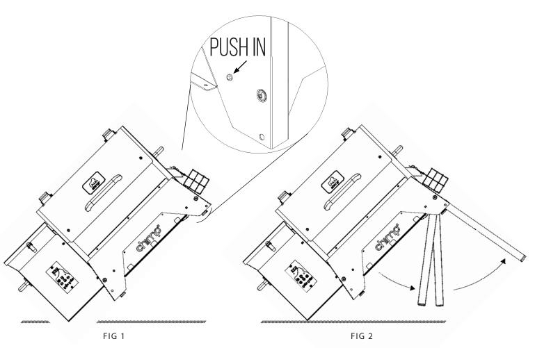
STEP 1 - Tilt grill up on the hopper edge illustrated in (FIG 1). Push in the metal detent on each side of the grill to release the two non-wheel legs (FIG 2). Make sure the detent clicks back into the downward postion holes.
