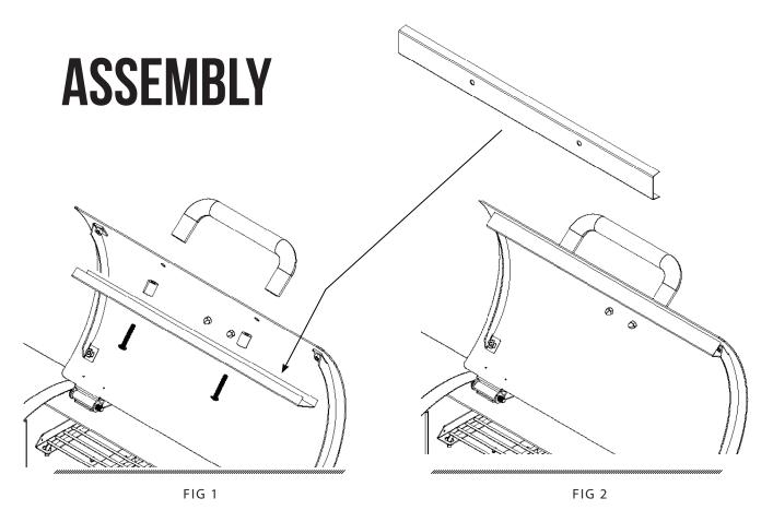
STEP 1 - Using the 2 longer 1/4" philips head screws supplied and the aluminum spacer. Mount the smoke deflector and lid handle to the stainless steel lid.
