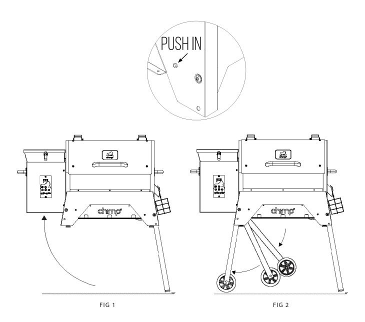
STEP 2 - Now lift hopper side using the handle on the hopper (FIG 1). Again push the metal detents on both sides of your grill to release the wheel legs, click them into place (FIG 2).
