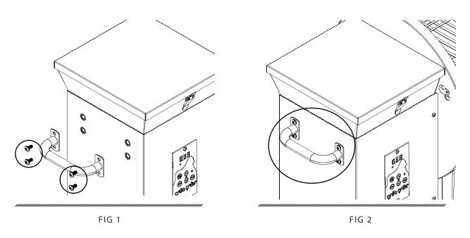
STEP 1 - Use the 4 shorter 1/4" philips head screws circled in FIG 1 to mount the hopper handle, Seen in FIG 2.
