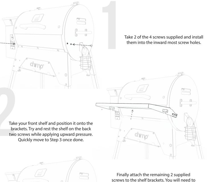
screws to the shelf brackets. You will need to adjust the shelf up and down a bit to allow the screws to feed through the slots and the bracket. Once in place tighten down.
