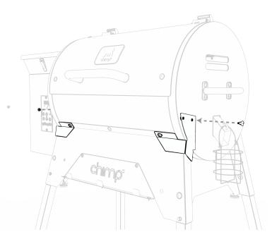
Once the brackets are in place, take 2 of the 4 screws supplied and install them into the inward most screw holes.
